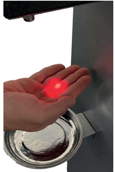
Sensor light spot navigates the hand to the correct positioning
