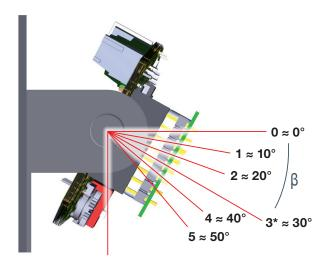
All settings are done as described in chapter 4.3 refer to the default setting with the click position setting 3 (approx.  $30^{\circ}$ , angle  $\beta$ ). Different click position settings must be tested individually on site.
