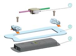
(1) sCON-S System connector 2 Door cover (3) Installed sensor
