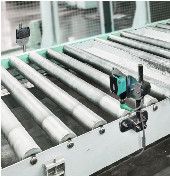
Conventional: Sensors above the conveyor
