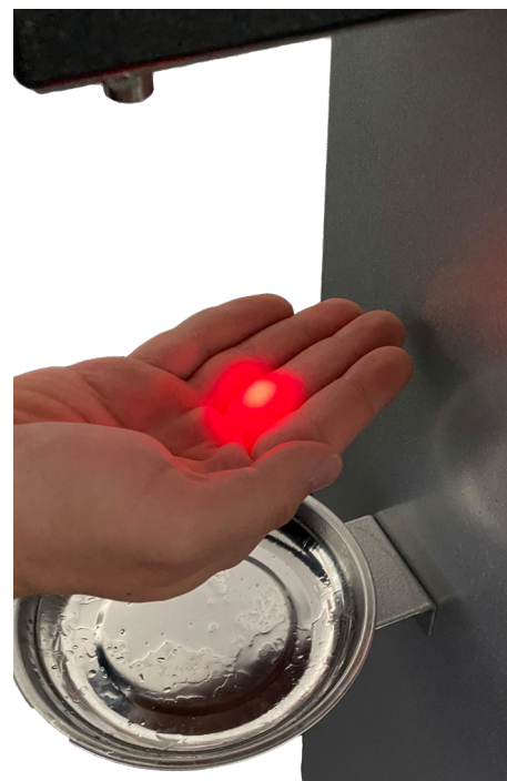
Sensor light spot navigates the hand to the correct positioning
