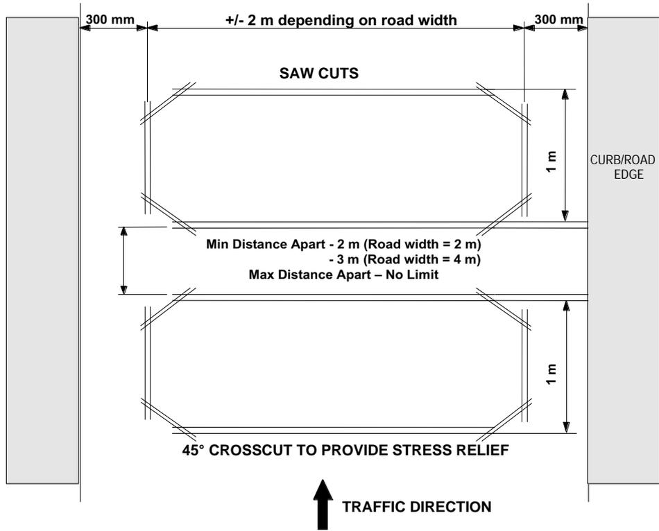
Figure 6. Adjacent loops connected to different detector modules
